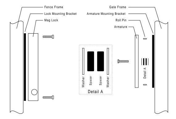
In some applications, the magnetic lock and/or the armature plate can be mounted without using the supplied mounting plates.
