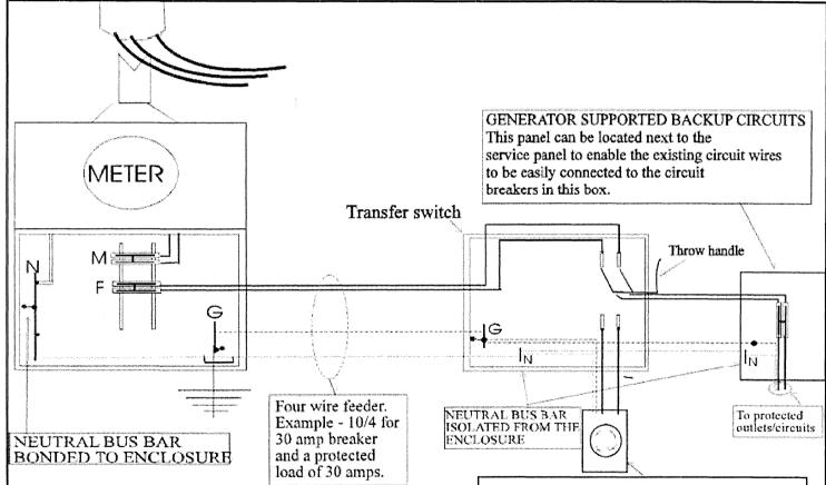
The generator needs to be located outside to avoid asphyxiation or listed by an approved agency for other locations. Proper installation is a critical safety issue that includes preventing back-feeding into the utility
